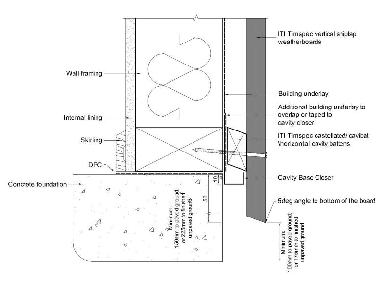
VC 501 Base, Concrete Slab on Ground
