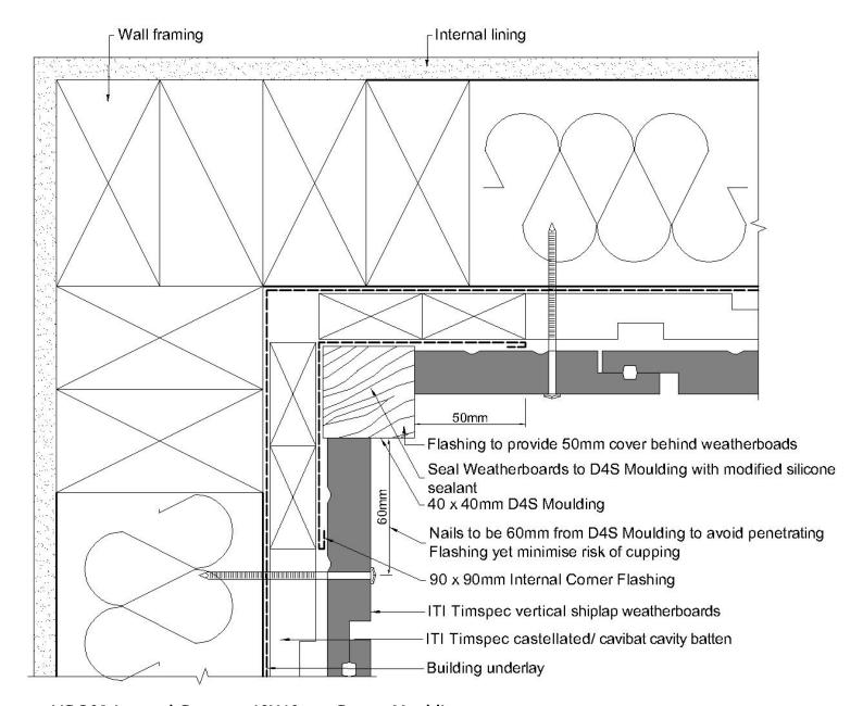
VC 301 Internal Corner - 40X40mm Corner Moulding
