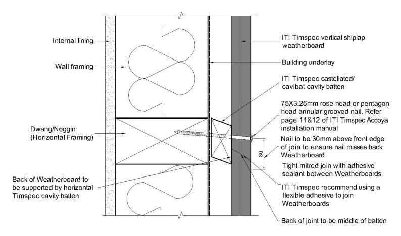
VC 402 Within Board Joint - Scarf Joint
