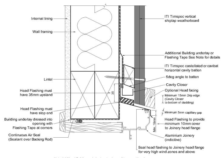
Note: Additional Building underlay to extend up wall to nearest lap above and extend down as far as possible into Cavity Closer.
