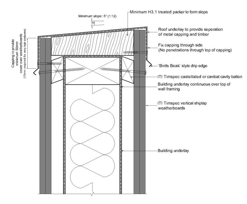
VC 701 Parapet Capping Expansion Joint
